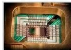
Photograph of a chip constructed by D-Wave Systems Inc. Mounted and wire-bonded in a sample holder. The D-Wave processor is designed to use 128 superconducting logic elements that exhibit controllable and tunable coupling to perform operations.
